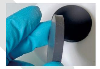
Made up of more than 90% cellulose, they are particularly suitable for samples requiring intense grinding. The XR-tab tablets playing the initial role of a grinding aid and secondly as a binding agent to obtain stable and resistant powder pressing tablets ready to introduce into the spectrometer in total confidence.
